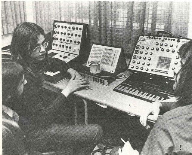
Fanshawe students working with synthesizer, pitch-to voltage convertor and computer sound generator.
